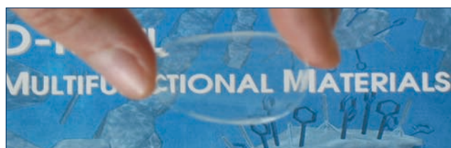
Photograph of a self-supporting and transparent polymethylmethacrylate film with 1 vol% titania nanoparticles.
